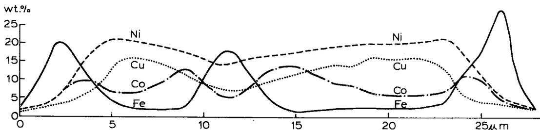
FIG. 2. Concentration profile across zoned crystals of disulfide from Karniowice.
