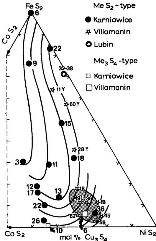
FIG. 1. Compositions of the Cu-Ni-Fe-Co disulfides. Numbers and contours indicate  $\text{CuS}_2$  content calculated on the bases of  $\text{Cu} + \text{Ni} + \text{Fe} + \text{Co} = 1$  and  $\text{Ni} + \text{Fe} + \text{Co} = 1$ . Sources: Karniowice: this study, Lubin: Moh & Kucha (1980), Villamanin: (dotted field) Maaskant (1968), (Y) Ypma *et al.* (1968), (L) La Iglesia *et al.* (1974).
