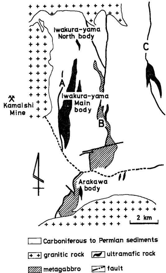
FIG. 2. Distribution of ultramafic rocks in the Kamaishi mining district, northeastern Japan. A: the Iwakura-yama tectonic line, B: the Ninokura-yama tectonic line, C: the Kogawa tectonic line.
