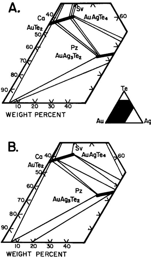
FIG. 9. Relationships in the synthetic Au-Ag-Te system. A represents the 300°C isotherm from Markham (1960), whereas B represents the 290°C isotherm from Cabri (1965). Abbreviations: (Ca) calaverite, (Sv) sylvanite, and (Pz) petzite.
