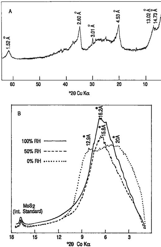
FIG. 2. X-ray-diffraction patterns of palagonite. A. Normal XRD. B. Low-angle XRD.
