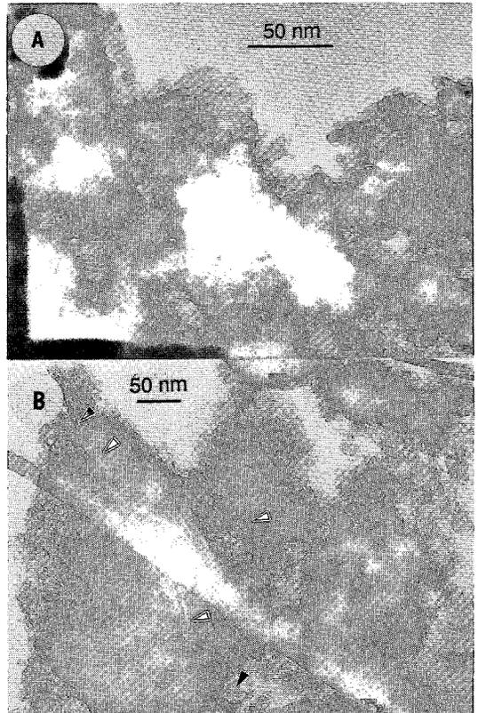
FIG. 5. Spheroidal particles in palagonite (A) and their replacement by randomly oriented short line-structures (arrows) (B).
