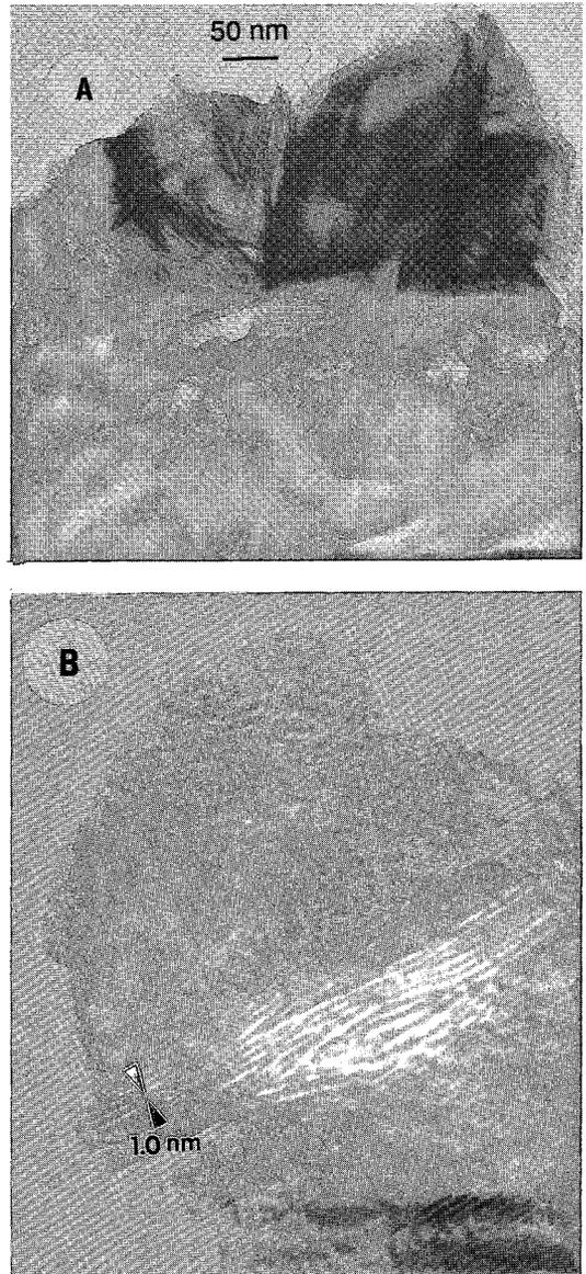
FIG. 3. Transmission electron micrograph (A) and lattice image (B) of the smectite-like particles in palagonite.
