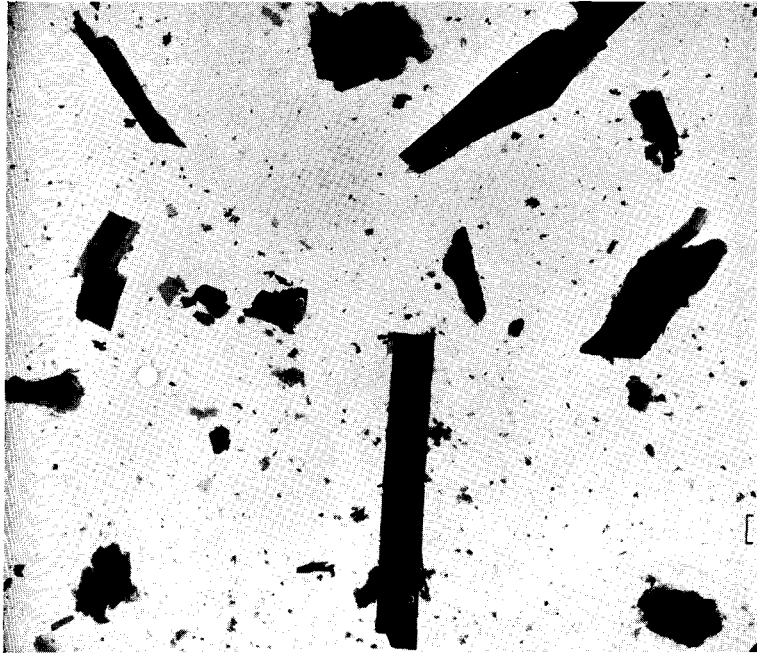
FIG. 3. Electron micrograph of mountainite showing rectangular laths with elongation b and principal cleavage (001). \times 4\,000 .
