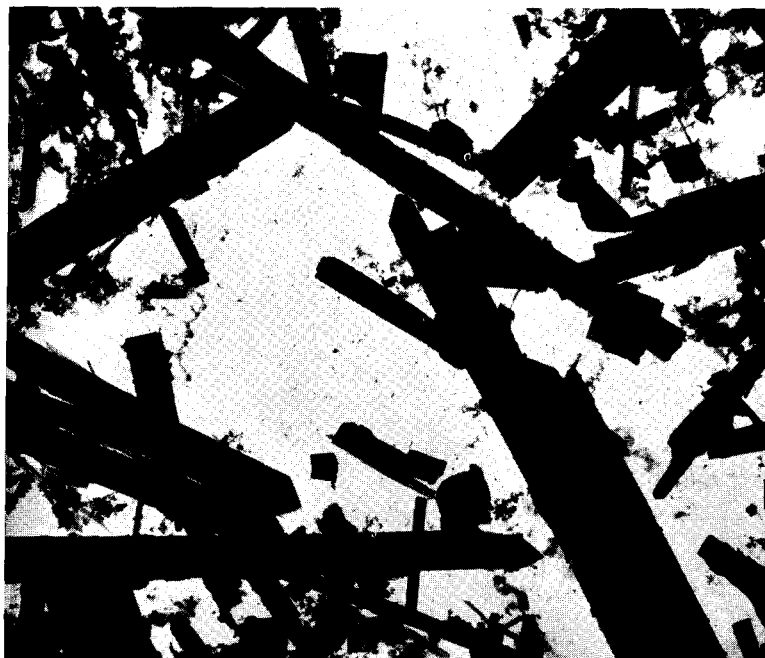
FIG. 1. Electron micrograph of rhodesite, showing laths with elongation c and principal cleavage (100). Some crystals have one end pointed. \times 4\,000 .
