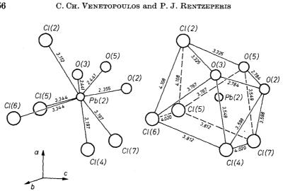
Fig.3. Clinographic projection of the coordination polyhedron around the atom Pb(2) of Fig.2
