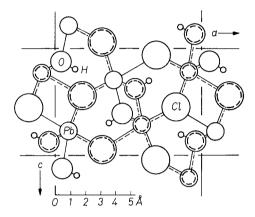
Fig.1. Projection of the structure parallel to b. Single full circles represent atoms at  $\frac{1}{4}b$ , whereas the double circles represent two atoms, one at  $-\frac{1}{4}b$  and one at  $\frac{3}{4}b$ . The atoms of the asymmetric unit are indicated with their symbols
