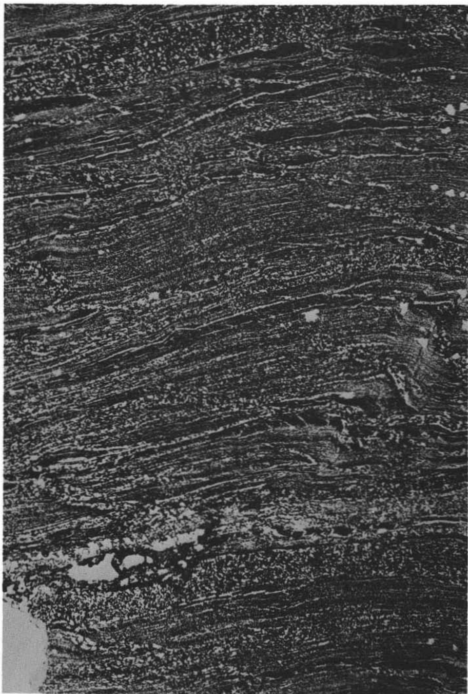
Fig. 7. — Thin section of «Massello Pietra» ; 1 Nicol, X 8 (about). - Cassiterite is black; the white thin seams/veinlets and the smallest white specks are made of Quartz aggregates, holding Tourmaline; this latter is not visible at this enlargement. Quartz, in some seams, in evidently pseudomorphous after rhomboedral minerals (probably Calcite). The large white spots (specially
