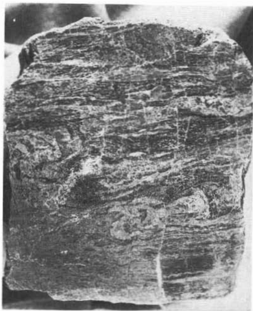
Fig. 14. — Ore-bearing horizon made up of garnets, epidotes, quartz. The sulphides are finely disseminated in the rock. Crystallization broadly synchronous with the microfolds are visible. S. Gabriele stope (Funtana Raminosa).
