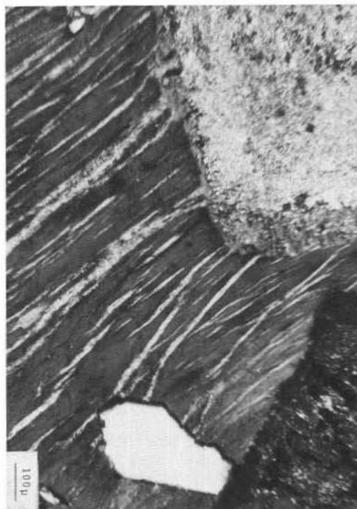
Fig. 3. — Argillic alteration; fresh perthitic K-feldspar crystal in contact with completely altered plagioclase crystals (Flumini Binu).
