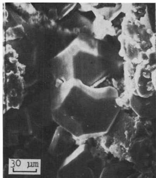
Fig. 6. — \text{NH}_4(\text{Cl}_{0.96}\text{Br}_{0.04}) {111} + {100} dendrite, \langle 100 \rangle orientation.
