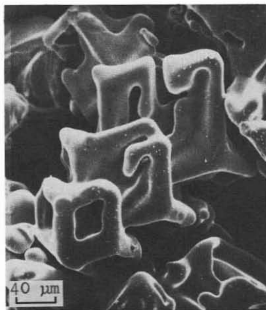
Fig. 8. — \text{NH}_4(\text{Cl}_{0.98}\text{Br}_{0.02}) \{110\} dendrite, \langle 100 \rangle orientation with initial \langle 111 \rangle protrusion.
