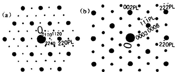
Fig. 3. Electron diffraction patterns of hongshiite.
