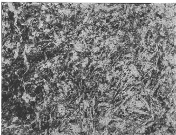
FIG. 3. Fused wood-ash stone, Grand Canyon National Park, Arizona. Shows fairchildite largely replaced by buetschliite and calcite, which retain the form of the original fairchildite. \times 30 ordinary light.
