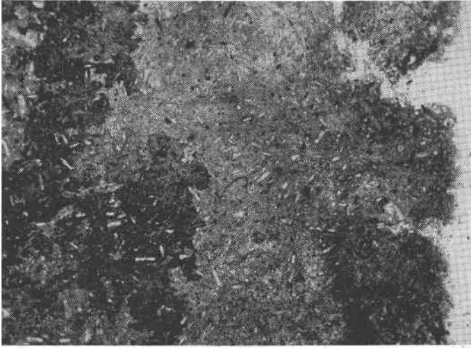
FIG. 4. Fused wood-ash stone Grand Canyon National Park, Arizona. This section was ground with water instead of oil; under these conditions decomposition of the fairchildite has produced buetschliite and calcite. The buetschliite has crystallized in characteristic stubby barrel-shaped crystals. \times 30 ordinary light.
