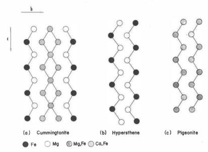
Fig. 3. Schemesof  $Mg^{2+}$ — $Fe^{2+}$  ordering in (a) cummingtonite—three dimensional section of the structure parallel to bc at x=0. (b) hypersthene—three dimensional section through the structure parallel to bc at x=0.125. (c) pigeonite—three dimensional section through the structure parallel to bc at  $x\sim0.25$ .
