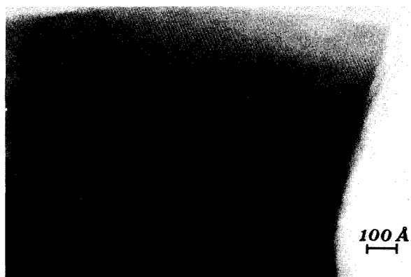
Fig. 4. Heavily disordered sequence of versiliaite ( 12\text{\AA} lattice fringes) and apuanite ( 9\text{\AA} lattice fringes) lamellae.
