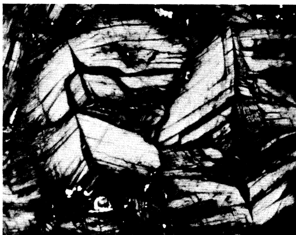
Fig. 2. Coyoteite crystals showing chevron pattern developed by opposing cleavage sets. Continuous parallel lines are polishing scratches. The long dimension of the photograph is 0.26 mm.
