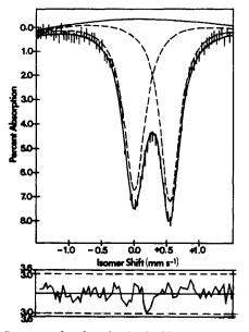
Fig. 5. Computer fit of a simple doublet to the Mössbauer spectrum of  $FeNi_2S_4$ .
