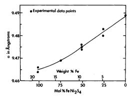
Fig. 2. Variation in unit cell parameter (a) with composition between  $FeNi_2S_4$  and  $Ni_3S_4$ . The unit cell parameter of  $Fe_3S_4$  is 9.876Å.
