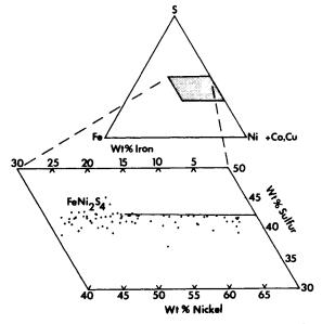
Fig. 8. Compositions of natural iron-nickel thiospinels shown in terms of Fe, Ni and S content (for sources of data, see Table 2).
