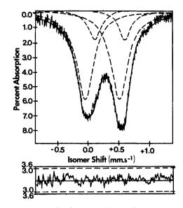
Fig. 6. Computer fit of two doublets to the Mössbauer spectrum of  $FeNi_2S_4$ .
