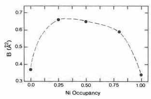
Fig. 3. Variation in M(1)-site isotropic displacement factors (B) with Ni occupancy at the M(1) site. M(1) occupancies were fixed at nominal values; all other structural and pattern parameters [except M(1) displacement factors] were fixed at values from the final overall refinements.
