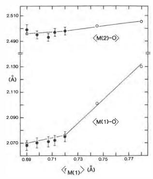
Fig. 6. Variation in  $\langle M(1)-O \rangle$  and  $\langle M(2)-O \rangle$  with mean ionic radius of the constituent cations at the M(1) site. Symbols are analogous to Figure 4.
