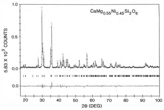
Fig. 1. Observed and calculated X-ray powder diffraction pattern for sample  $Ni_{50}$  (CaMg<sub>0.55</sub> $Ni_{0.45}Si_2O_6$ ). The crosses are the observed data, the solid line is the calculated pattern, and the vertical bars mark all possible Bragg reflections ( $K\alpha_1$  and  $K\alpha_2$ ). The difference between the observed and calculated patterns is shown at the bottom.
