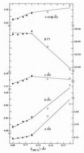
Fig. 4. Variation in cell parameters a, b, c,  $\beta$  and c sin  $\beta$  with mean ionic radius of the constituent cations at the M(1) site (solid circles). Open circles are data from the single-crystal structures of CaNiSi<sub>2</sub>O<sub>6</sub> and CaCoSi<sub>2</sub>O<sub>6</sub> (Ghose et al., 1987), diopside (Levien and Prewitt, 1981), and hedenbergite (Clark et al., 1969).
