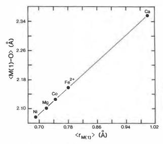
Fig. 7. Variation in (M(1)-O) with constituent cation radius in synthetic ordered olivines. Ni<sub>2</sub>SiO<sub>4</sub>: Brown (1970); Mg<sub>2</sub>SiO<sub>4</sub>: Hazen (1976); Co<sub>2</sub>SiO<sub>4</sub>: Morimoto et al. (1974); Fe<sub>2</sub>SiO<sub>4</sub>: Hazen (1977); Ca<sub>2</sub>SiO<sub>4</sub>: Smith et al. (1965).
