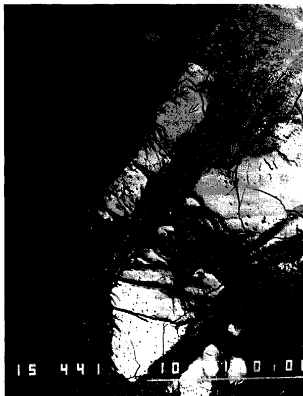
FIGURE 3. Backscattered electron image of relict uraninite (bright contrast) partly replaced by clarkeite and K-rich phase (darkest contrast). Bubbles in the uraninite are preserved in the surrounding clarkeite (arrows), suggesting solid-state replacement (sample DMNH 13283). Scale bar at lower right is 100 \mu\text{m} .
