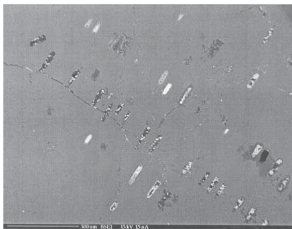
FIGURE 2. BSE image showing solid and melt inclusions within the kaersutite. White color within the inclusion is pyrrhotite; dark gray is hematite; light gray is magnetite.
