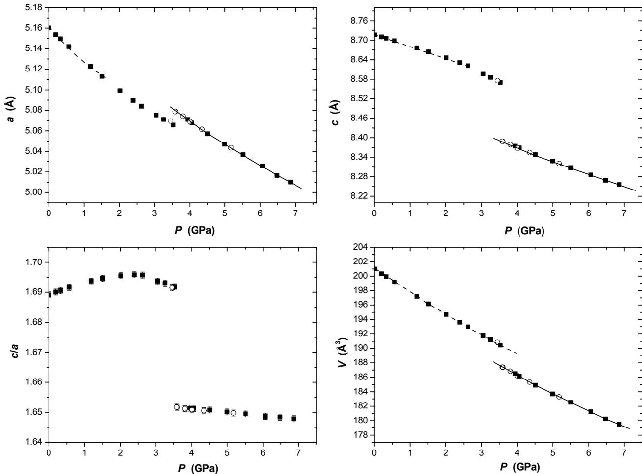
FIGURE 2. Variation of the unit-cell parameters of kalsilite with pressure. Open symbols represent data collected in decompression. The dashed and solid lines represent the axial and volume third-order Birch-Murnaghan EoS fits for the low- $P$  and high- $P$  polymorphs, respectively. The e.s.d. values are slightly smaller than the size of the symbols.
