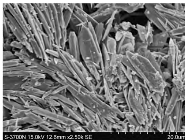
FIGURE 2. Minute pseudojohannite crystals on PIP 1/2000 holotype specimen, from Jáchymov deposited in collections of the National Museum in Prague. SE image by J. Sejkora (Hitachi S-3700N).
