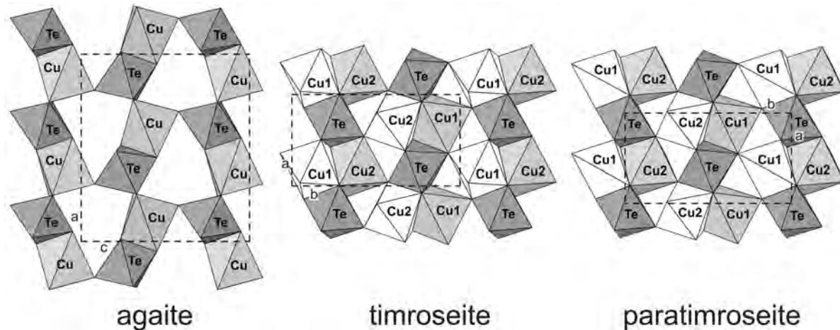
**FIGURE 3.** The polyhedral sheets in the structures of agaite, timroseite, and paratimroseite. The sheets are essentially the same, if the unshaded CuO<sub>5</sub> and CuO<sub>6</sub> polyhedra in the sheets in timroseite and paratimroseite are ignored.
