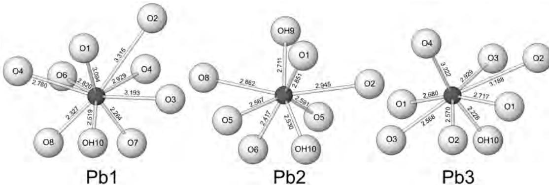
**FIGURE 4.** Pb coordinations in agaite. The lopsided distributions of bond lengths are attributable to the localization of the lone-pair electrons. Bond lengths are given in angstroms.
