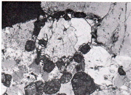
Fig. 3. Altered, nearly isotropic zircon crystals (dark gray) surrounding larger monazite crystals (light gray). The medium gray mineral is plagioclase. Oblique nicols. Magn. 130 \times .
