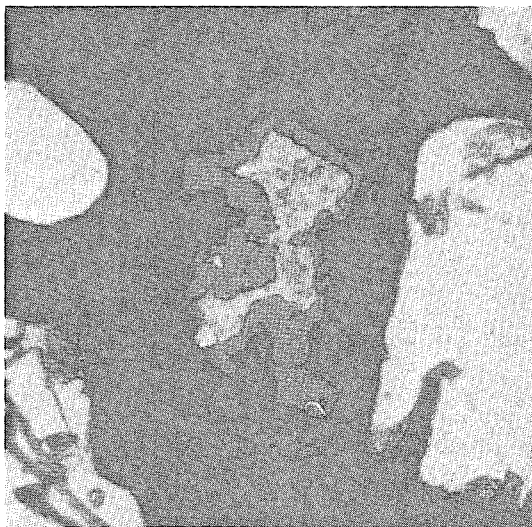
FIG. 3. Irregular gold grain with coating of limonite (x 720).
