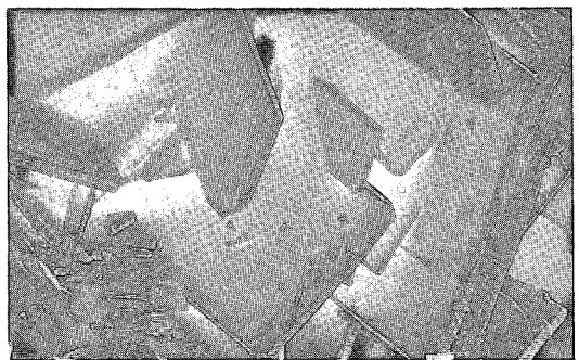
FIG. 6. Thin lamellae of parascholzite in a radiating arrangement. Time elapsed since implantation: 13 years. Scale bar: 10\text{ }\mu\text{m} .
