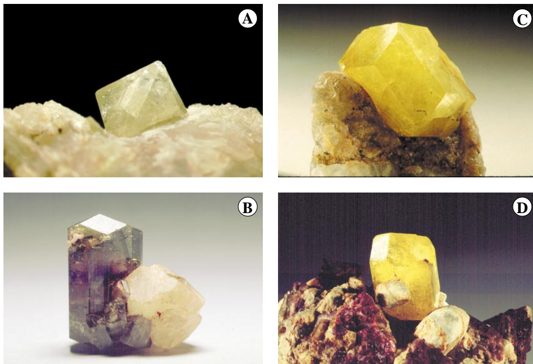
FIG. 2. Color photographs of the londonite crystals. A. A pale yellow-green crystal of londonite on saccharoidal albite from the Antandrokomby pegmatite, Madagascar. The crystal is 0.7 cm across and shows dodecahedron {110}, tristetrahedron {211}, and tetrahedron {111} faces (photo by R. Appiani). B. Milky pale yellow crystal of londonite (1 cm) on a crystal of liddicoatite from Ampanivana, Madagascar (photo by R. Appiani). C. Large, well-formed dodecahedral, sulfur-yellow londonite crystal (1.8 cm) from Antsongombato, Madagascar (photo by W. Wilson). D. An exceptionally large, gemmy, sulfur-yellow londonite crystal (3.5 cm) from Antsongombato, Madagascar (photo by F. Valoti).
