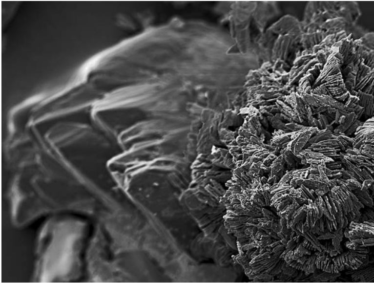
FIG. 1. Two types of zippeite crystals. In the background, the older zippeite, studied by SC-XRD. The younger zippeite (right, focused part of the image) locally covers the massive crystalline aggregates. SE image, field of view 250 \mu\text{m} (JEOL JSM-6380).
