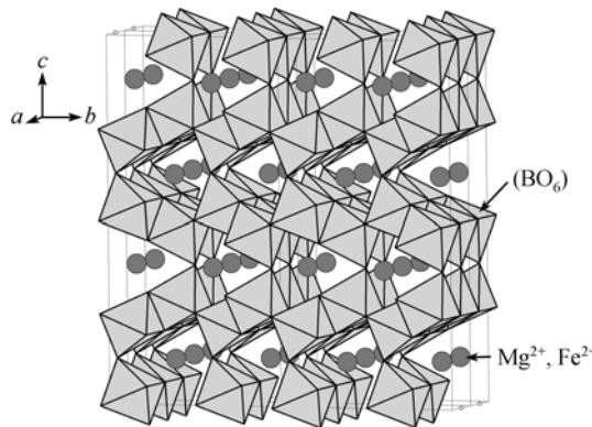
**Figure 4** Schematic view of xieite structure showing that  $\text{Cr}^{3+}$  and  $\text{Al}^{3+}$  occupy octahedral sites ( $\text{BO}_6$ ), whereas  $\text{Mg}^{2+}$  and  $\text{Fe}^{2+}$  occupy dodecahedral sites.
