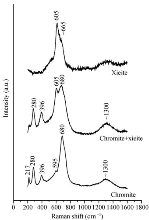
**Figure 2** Raman spectra showing xieite, chromite and a mixture consisting of both chromite and xieite. The upper is a xieite spectrum recorded from a polycrystalline aggregate of xieite occurring within a shock vein. The lower is a chromite spectrum measured from a chromite grain in the chondritic portion apart from the shock veins. The middle is a mixture spectrum from chromite plus xieite obtained from a chromite grain with lamellar texture in chondritic portion adjacent to a shock vein.
