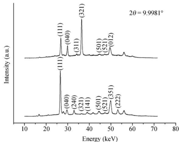
**Figure 3** X-ray diffraction patterns of polycrystalline aggregate of xieite obtained from two different orientations of the sample. The numbers listed at diffraction peaks are the Miller indices representative of the orientation of atomic planes in a crystal lattice.
