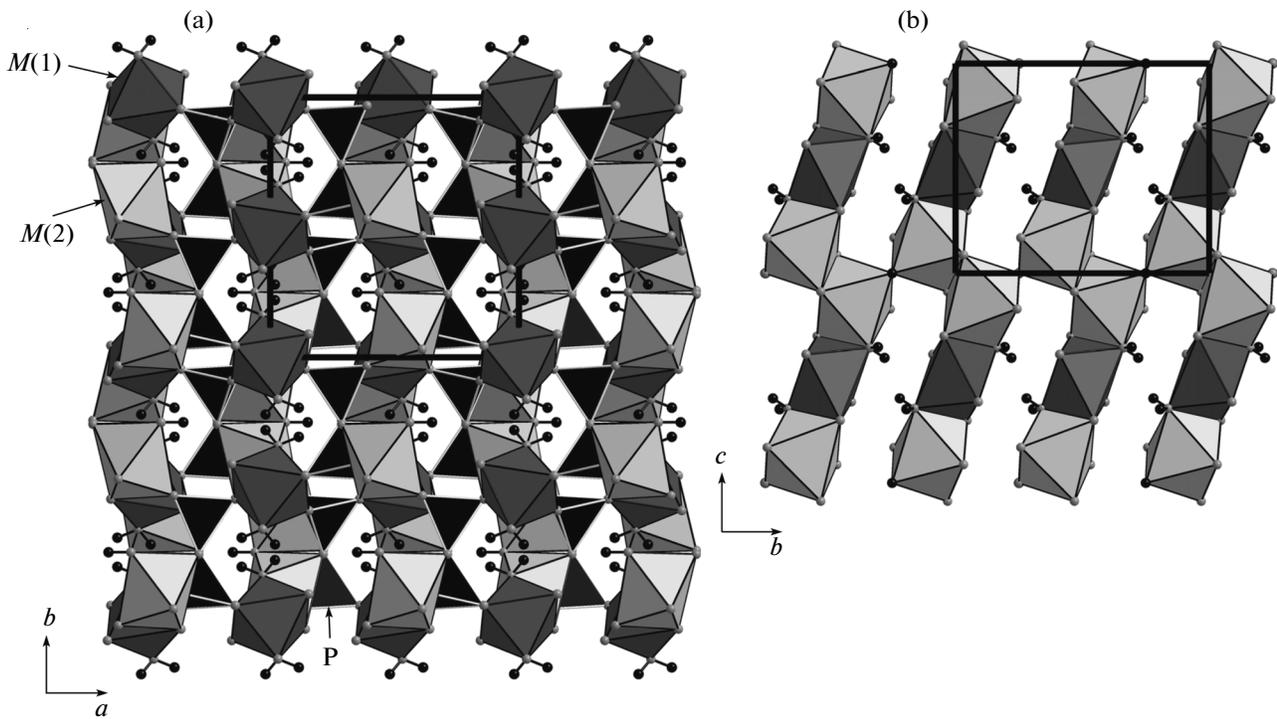
**Fig. 1.** Crystal structure of garyansellite (a) and the layer of *M*(1) and *M*(2) centered octahedra (b). Oxygen atoms are shown by gray circles; hydrogen atoms are shown by black circles. Unit cell is shown.
