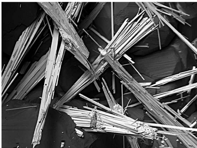
Fig. 2. SEM image of fibres of mo loite. The horizontal length of the photograph corresponds to 3 mm.
