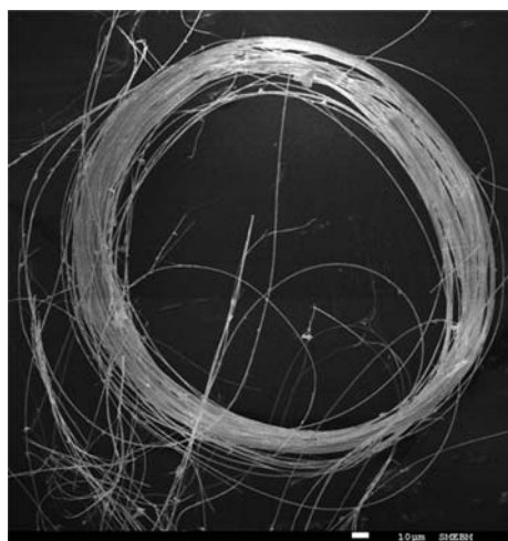
Fig. 7. SEM image of a nest-like wire of the fibrous habit of tubulite (Biò).
