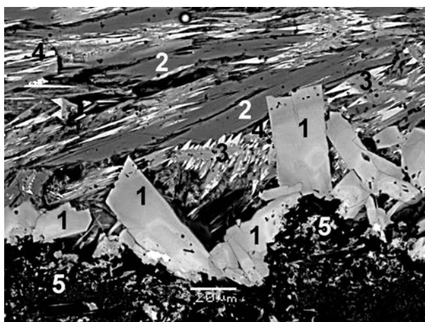
Fig. 4. Assemblage of vanadium minerals (1–4) on the basalt scoria matrix (5): 1–grigorievite, 2–bannermanite, 3 and 4–epitactic(?), dendritic aggregates of two uncharacterized Ca–Cu vanadates. Polished section, SEM (BSE) image. Field of view: 0.18 mm.
