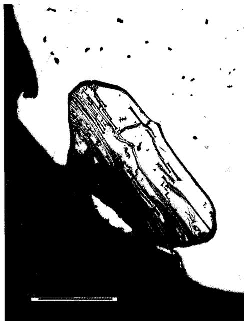
Fig. 5. Polished section of a platinum grain (light grey), including luberoite (dark grey). The latter, located at the border of the platinum, displays cleavages filled with anatase. Reflecting light microscope, unpolarized light, oil immersion. Scale bar = 100  $\mu\text{m}$ .
