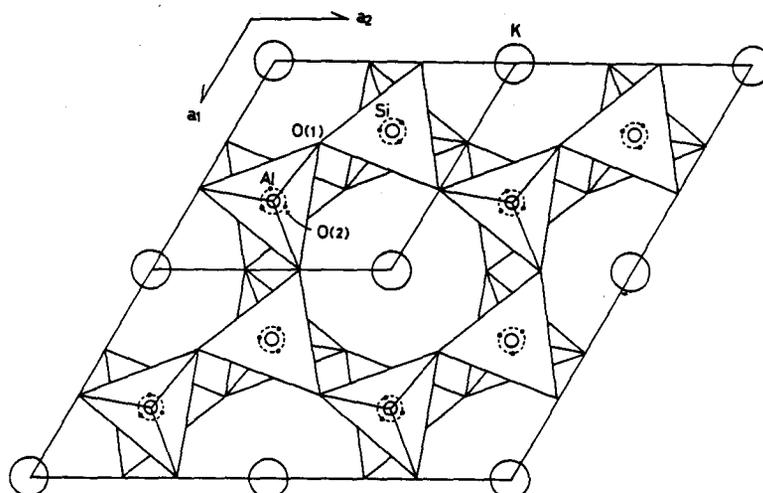
FIG. 1. The (001) projection of the structure of synthetic kalsilite. Each tetrahedron is connected by three O(1) atoms in the plane perpendicular to the  $c$ -axis and by one O(2) atoms in the direction parallel to the  $c$ -axis. O(2) atoms are distributed into three different positions near triad axis as shown by the dotted line in the figure.
