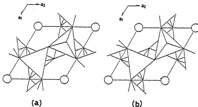
FIG. 2. Schema of the positional relationship of the domain structure. The structure has two types, (a) and (b), and these are related by mirror planes through longer diagonal of the unit cell.
