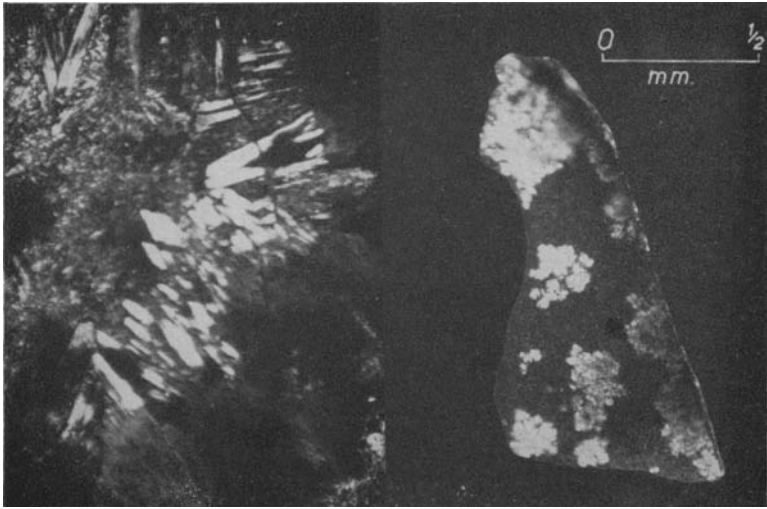
FIG. 2 ( left ). Acicular mesolite terminating in birefringent paddle-shaped crystals penetrating tobermorite, Portree, Isle of Skye. Crossed nicols, \times 44 (B.M. 1961, 162). FIG. 3 ( right ). Tacharanite, almost isotropic, with inclusions of birefringent gyrolite, fragment, Portree, Isle of Skye. Crossed nicols, \times 50 (B.M. 1961, 163).
