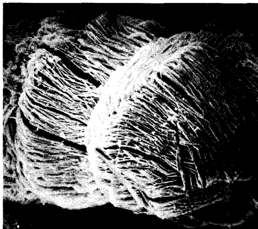
FIG. 1. Nodular ranunculite showing the aggregates of lamellar crystals (Scanning electron photograph, \times 800 ).
