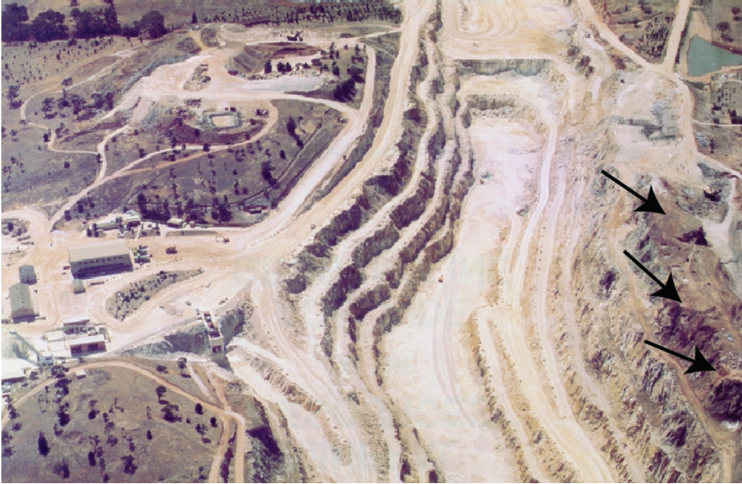
FIG. 2. Aerial photograph of the Penrice marble quarry in the late 1980s, showing the dark-brown phosphate zone (arrowed) above the marble. Photograph courtesy of Vince Peisley.
