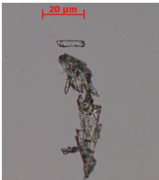
FIG. 3. Extremely thin and small crystals of deveroite-(Ce) from the holotype (top of the figure). The crystal was used to obtain the optical properties and the single-crystal data by synchrotron radiation
