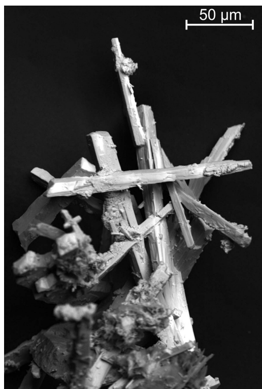
FIG. 1. Backscatter scanning electron microscope image of torrecillasite crystals.
