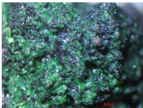
FIG. 2. Black, coarsely crystalline crust of melanarsite partially overgrown by bright green dmisokolovite. Field of view: 5.9 mm. Photo: I.V. Pekov and A.V. Kasatkin.
