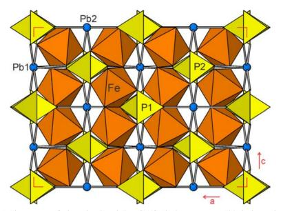
FIG. 5. The structure of crimsonite viewed along [010]. The low-occupancy Pb3 site is not shown.
