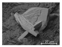
FIG. 2. Electron back-scatter scanning electron micrscope image of crimsonite crystals on plumbogummite. NHMLAC specimen number 65558.
