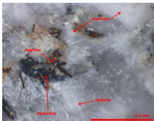
FIG. 1. Loose aggregates of nolzeite with nepheline, aegirine and analcime.
