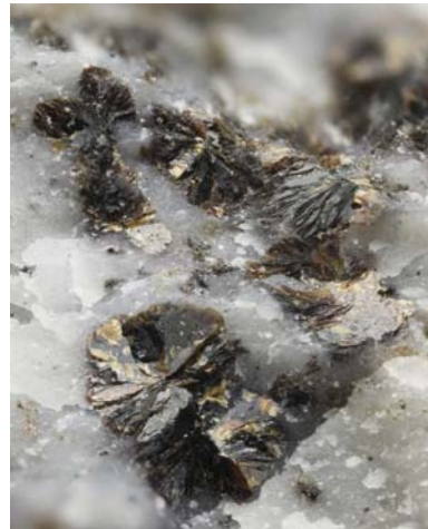
FIG. 1. Aggregates of radiating lath-shaped wicklundite crystals, showing typical very dark reddish brown colour and lustre. The fine-grained grey white matrix consists of manganiferous calcite. Field of view is 1.5 mm. Photo:
