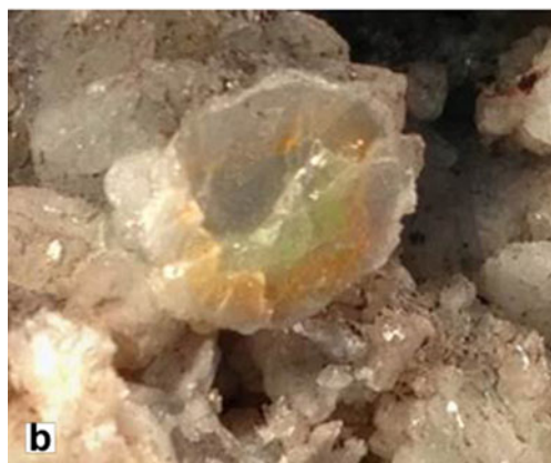
FIG. 1. (a) Somersetite crystal (green subhedral grain in the vug), field of view = 1 cm and (b) multi-coloured somersetite crystal (2 cm across) with inclusions of plumbonacrite and colourless transparent cerussite in the rim. The green zone is enriched in somersetite, but plumbonacrite was also determined from this area, whereas the white zone is enriched in plumbonacrite. All of these minerals can be identified reliably, by X-ray techniques.
