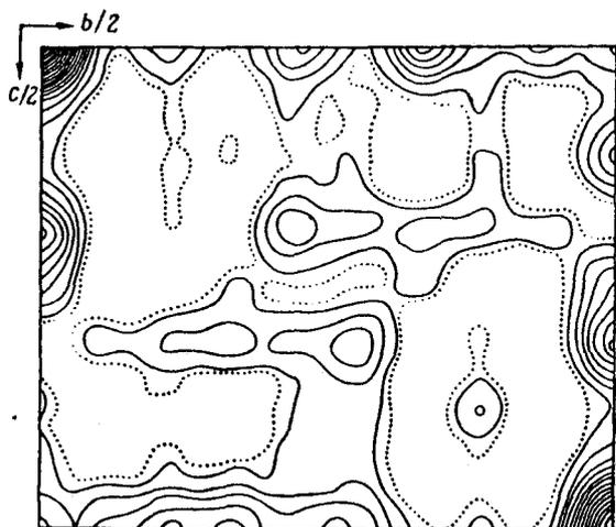
Fig. 1. Patterson projection on  $yz$  (one quadrant) for hurlbutite (paracelsian).
