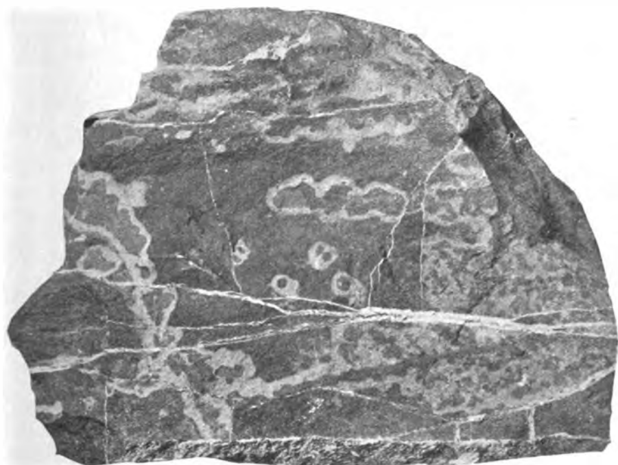
SANDSTONE IMPREGNATED WITH VANOXITE SHOWING PECULIAR BLOTCHING DUE TO SEGREGATION OF THE VANOXITE, JO DANDY MINE, PARADOX VALLEY, COLO.
