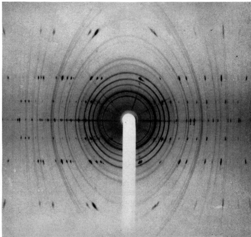
*c* axis oscillation pattern of lawsonite crystal from Blake Gardens after heating for 154 hours at 450°C. Cu radiation, Ni filter, 6-hour exposure.
