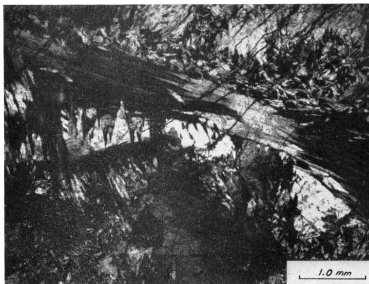
Fig. 2. Sheath of pumpellyite crystals in upper center of picture with "oak-leaf twins" below. Crossed nicols.
