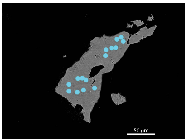
FIGURE 1. BSE image at 15 kV of giniite. Dots are locations of EMP analysis on the crystal. (Color online.)
