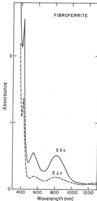
FIG. 5. Optical absorption spectrum of a bundle of fibroferrite fibers 250  $\mu m$  thick soaked in a liquid with  $n_D = 1.54$  (specimen from Cyprus).
