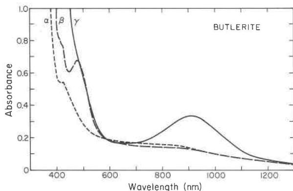
FIG. 3. Optical absorption spectrum of a butlerite crystal 106  $\mu\text{m}$  thick from Jerome, Arizona.
