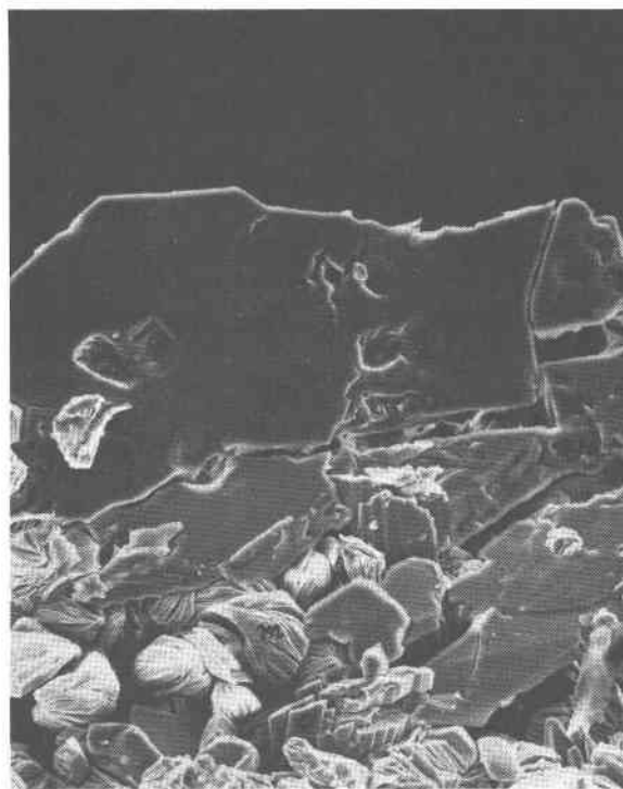
Fig. 3. Large (broken) crystal of abelsonite (a), with sheaves of an authigenic micaceous mineral (m), and orthoclase crystals (o) (Wosco). Scanning electron micrograph, 160 \times .
